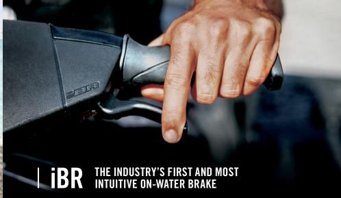
Recognized by the U.S. Coast Guard for improving boat safety since 2009 and now in its third generation, the Sea-Doo exclusive iBR (Intelligent Brake and Reverse) system allows you to stop up to 160 feet (48 m) sooner than watercraft not using a brake. With both hands on the handlebars, riders can engage forward, neutral, and reverse for stable, worry-free maneuvering at low speeds. \*Based on BRP internal testing.
