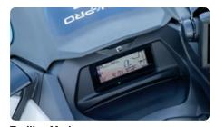
**Trolling Mode** Enables precise control of speed. Choose one of several pre-sets and adjust as needed.
