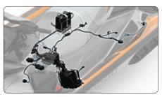
Advanced Battery System With dual batteries and a 650-watt voltage generator, even the most demanding electrical needs are sure to be met.
