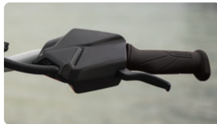
iBR® (Intelligent Brake & Reverse) Exclusive to Sea-Doo®, iBR® stops the watercraft sooner and provides more control and maneuverability at low speeds and in reverse.
